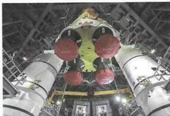
**SLS Core Stage Placed on Mobile Launcher**
