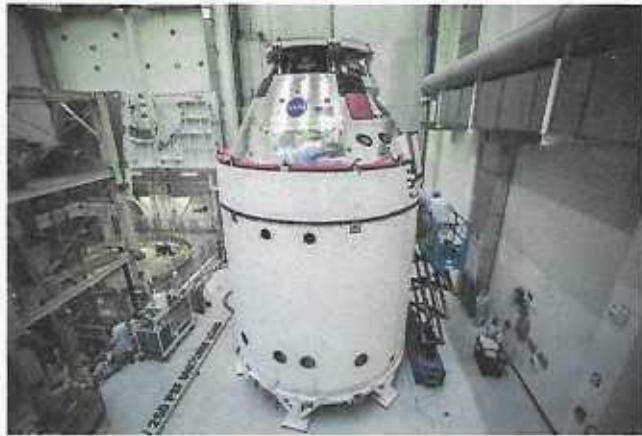
**Orion ESM Module Fitted With Jettison Fairing Panels**
