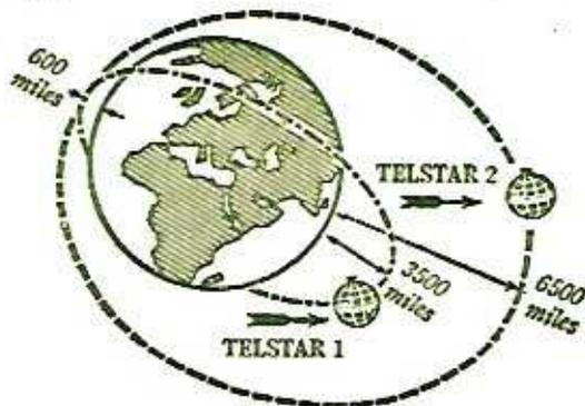
*TELSTAR 2 was projected deeper into space than TELSTAR 1, making possible longer transmission periods between the United States and Europe.*
