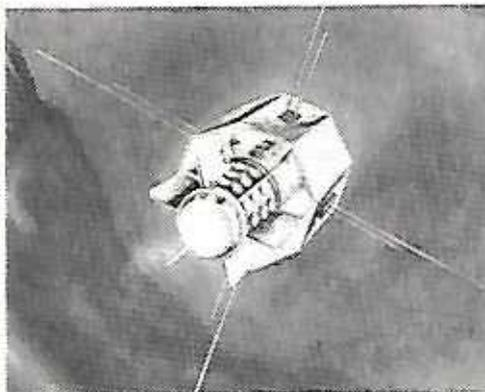
Navigation Satellite in orbit today from Vandenberg Air Force Base, California. To provide highly accurate Navigation systems for Polaris Submarines, Naval Ships, and Aircraft. First Satellite system to use an ATOMIC Power Source.
