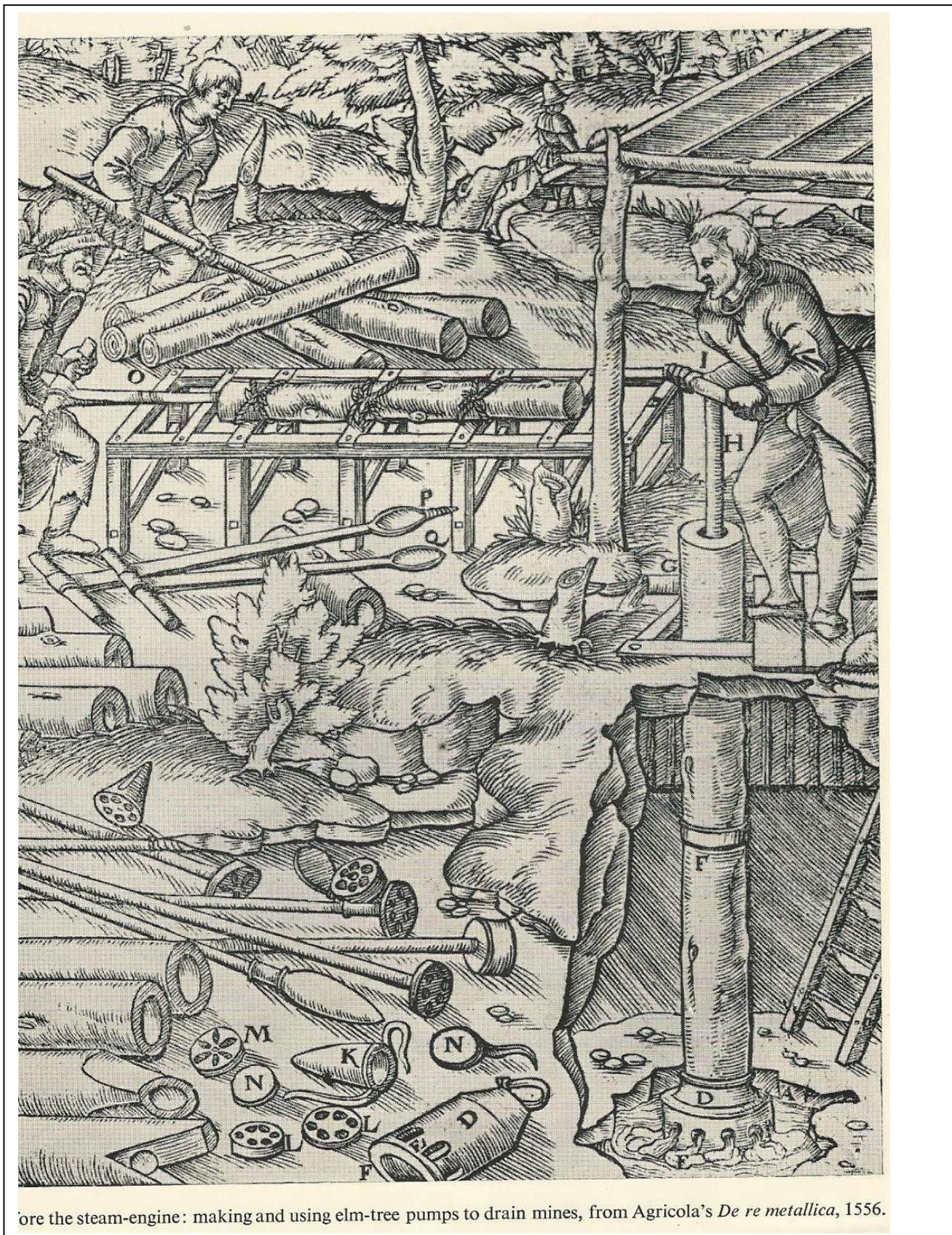
ore the steam-engine: making and using elm-tree pumps to drain mines, from Agricola's *De re metallica*, 1556.
