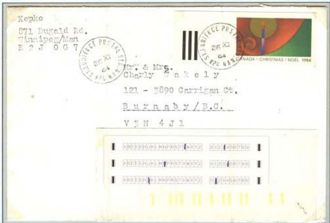
OCR sticker (Canada): allow senders to tick with a pen the postal code. This simplifies the OCR recognition and quicker sorting.
