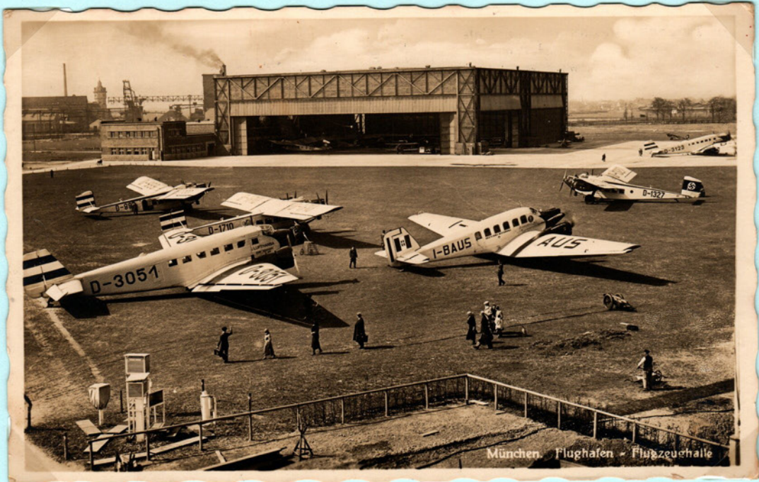
Munich airport was an important hub for the various airlines operating in Europe during the period. The postcard shows several aircraft, mostly Junkers, of Lufthansa, one of OLAG (bottom) and one of SAM, the three-engine Junkers G.24 I-BAUS, capable of accommodating up to 10 passengers.
