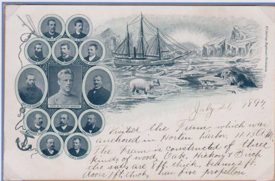
21/07/1897. Picture postcard depicting the members of the expedition with very interesting handwritten information about the technical details of the ship: "The Fram is constructed of three kinds of wood, oak, hickory and birsch."
